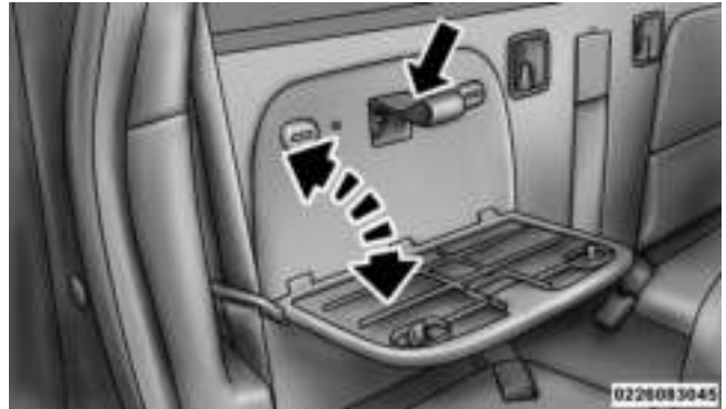
Rear Seat Tether Strap Routing Loop, Club Cab/Extended Cab (2005-2011 Model Years)
