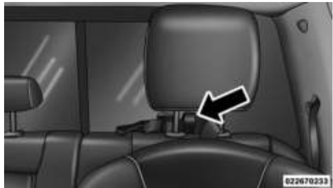
Tether Strap Through Outboard Tether Strap Loop
