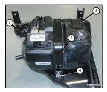
17. Remove the ground wire harness bolt (1).
