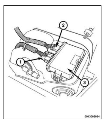
13. If necessary, remove the bolts (1) and the DEF pump cover (2).
