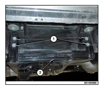
10. Remove left side bolts (1) and partially lower the DEF tank (2).
