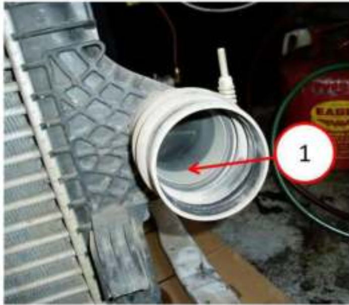
Fig. 4 CHARGE AIR COOLER INLET
