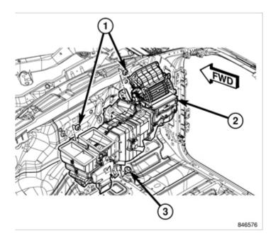
1. Position the HVAC housing assembly (2) into the passenger compartment and over the studs on the dash panel, with the condensate drain tube in its proper location.
