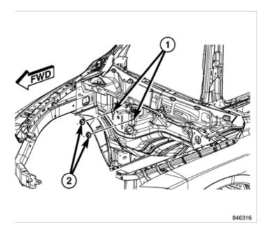
7. Install the two nuts (2) onto the two studs (1) that secure the HVAC housing to the engine compartment side of the dash panel. Tighten the nuts to 6.8 Nm (60 in. lbs.).
