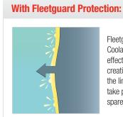
Fleetguard Fully Formulated Coolant can prevent the fatal effect on your engine by creating a protective layer on the liner wall: implosions now take place on this layer and spare the liner surface.
