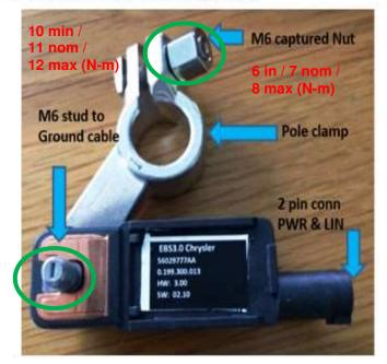
Battery Sensor 3.0 – 90 degree pole clamp
