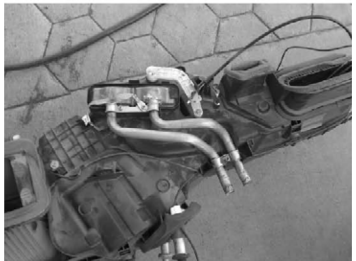
HVAC box removed from the truck. Heater core and attached pipes are approximately in the center.
