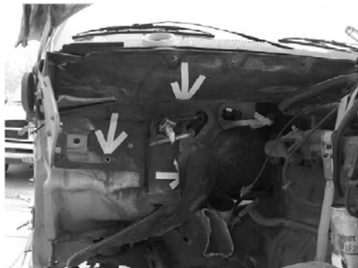
View under the hood of a partially disassembled truck. The positions of the four HVAC box mounting nuts are shown by arrows.
