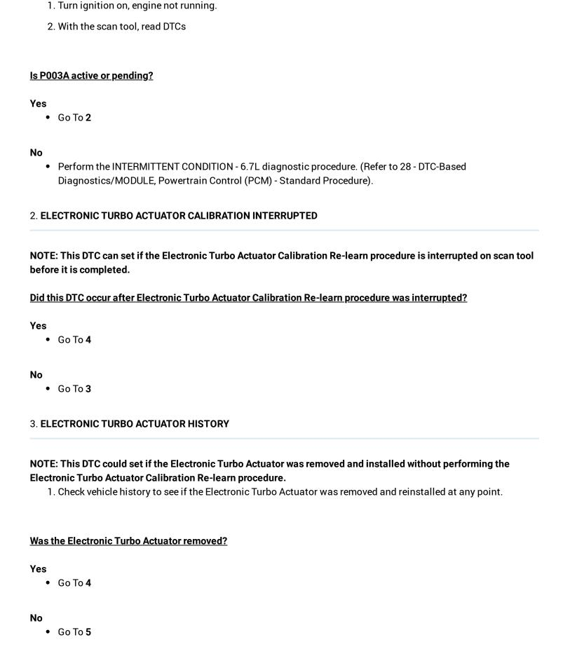
NOTE: If the Electronic Turbo Actuator Calibration procedure was recently performed, it could set this DTC.
