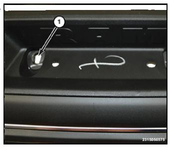
6. If equipped with the 115 V power outlet (2), remove the fastener (1) inside the lower right tray above the outlet.
