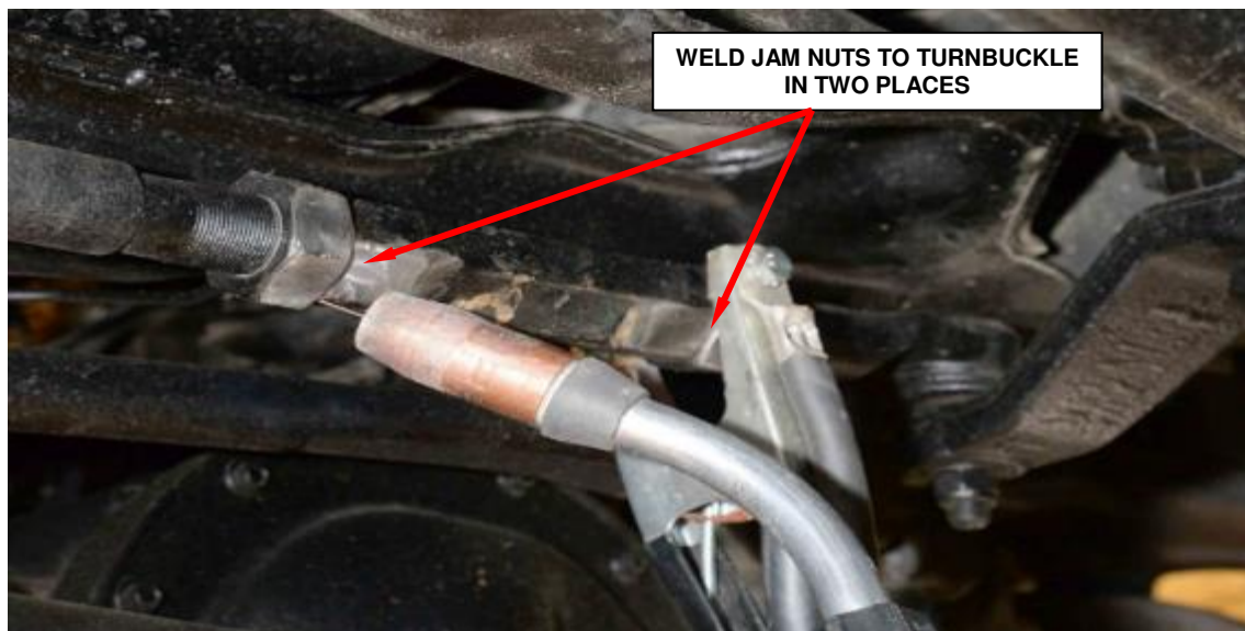
Figure 9 – Weld Both Jam Nuts to the Turnbuckle
