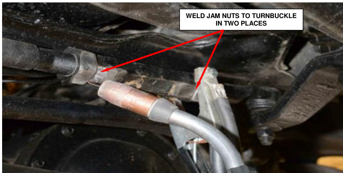
Figure 9 – Weld Both Jam Nuts to the Turnbuckle
