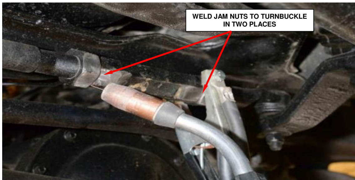
Figure 9 – Weld Both Jam Nuts to the Turnbuckle
