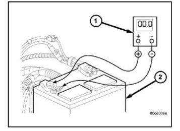
2. Connect positive lead of voltmeter to positive battery terminal post. Connect negative lead of voltmeter to battery positive cable clamp. Rotate and hold ignition switch in Start position. Observe voltmeter. If voltage is detected, correct poor contact between cable clamp and terminal post.
