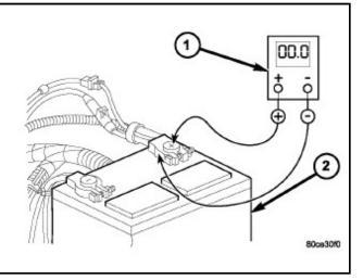
3. Connect voltmeter (2) to measure between positive terminal post on battery (1) and the battery terminal stud on the starter solenoid (3). Rotate and hold ignition switch in Start position. Observe voltmeter. If reading is above 0.2 volt, clean and tighten battery cable connection at solenoid and repeat test. If reading is still above 0.2 volt, replace the positive battery cable.
