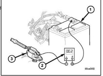
4. Connect voltmeter (1) to measure between negative terminal post on battery (2) and a good clean ground on engine block (3). Rotate and hold ignition switch in Start position. Observe voltmeter. If reading is above 0.2 volt, clean and tighten negative battery cable attachment on engine block and repeat test. If reading is still above 0.2 volt, replace the negative battery cable.
