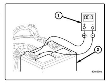
Connect positive lead of voltmeter to positive battery terminal post. Connect negative lead of voltmeter to battery positive cable clamp. Rotate and hold ignition switch in Start position. Observe voltmeter. If voltage is detected, correct poor contact between cable clamp and terminal post.
