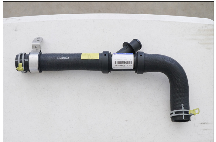
Upper radiator hose/Y-pipe assembly was one notable premature failure.
