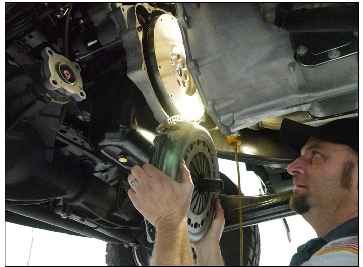
This South Bend Clutch and traditional flywheel in my 2017 Regular Cab will probably last longer than the factory dual-mass flywheel and my 2014 Crew Cab. Time will tell.
