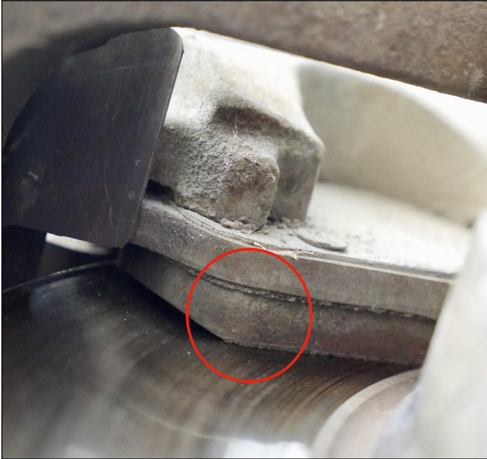
This is the front brake pad on my 1996 F-350 after 133,000 miles. Plenty of material remaining!
