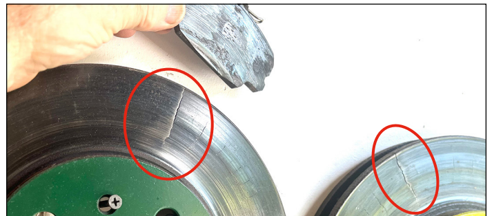
I thought I'd add a picture of a worn-out brake pad. Yep, it is a front brake pad from the E30 race car that was discussed on page 9. Yep, the rotors in the background are cracked-out. I've learned a lot about brakes!
