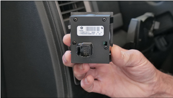
Newer vehicles can be easier to work on than older ones; this headlight switch assembly was a quick R&R.
