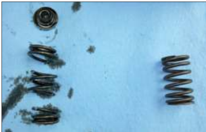
The valve spring retainer, broken valve spring and new spring on right.
