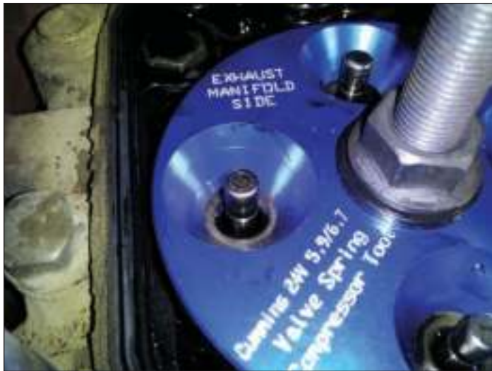
Close up of the compressed springs without the valve stem retainers.
