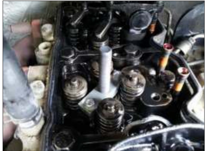
The injector hold down and both fasteners are removed so the base of the spring compressor can be installed. Since the injector is removed, it's simple to peer down into the cylinder. I told you that the piston is at TDC.
