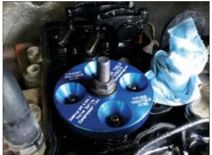
The push rods were checked and re-installed. Notice the rag covering the push rod openings? Why tempt fate with an errant valve stem retainer? The tool will smoothly depress the valve springs and stays centered on the springs. Keep a pencil magnet and a magnetic parts bowl handy to hold your parts.
