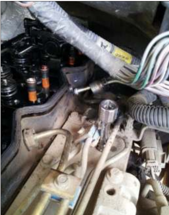
The tool requires the fuel injector to be removed. Notice the 3/8" drive extension holding the loosened fuel line away from the head so the connector tube can be disengaged from the injector inlet.
