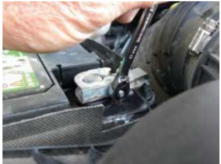
Loosen terminals with an 8mm box wrench; remove by twisting terminal with pliers.
