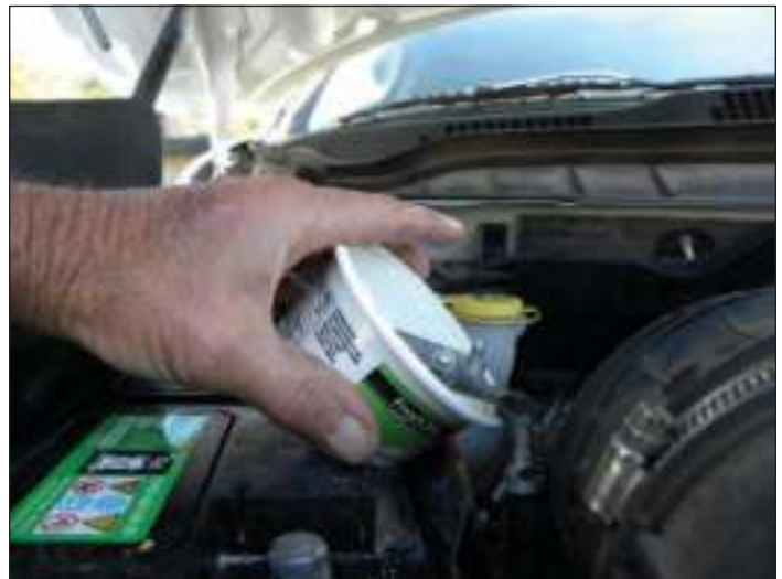
Soak terminal with a solution of 1/2tsp. of baking soda in water. Repeat twice.
