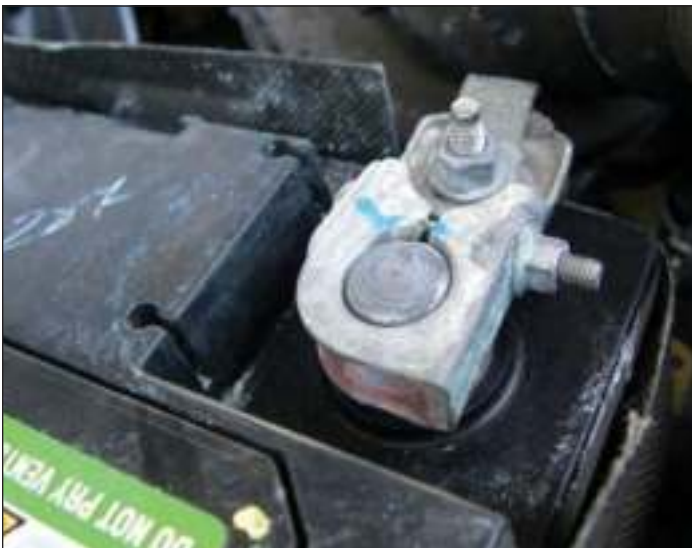
Slide terminal fully on post, tighten securely. Check for new corrosion in two weeks.
