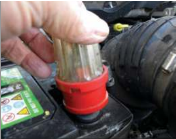
Clean battery post with a wire brush until shiny.
