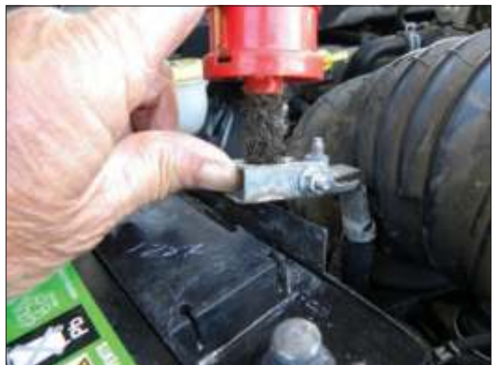
Wire brush terminal inside until shiny bright.
