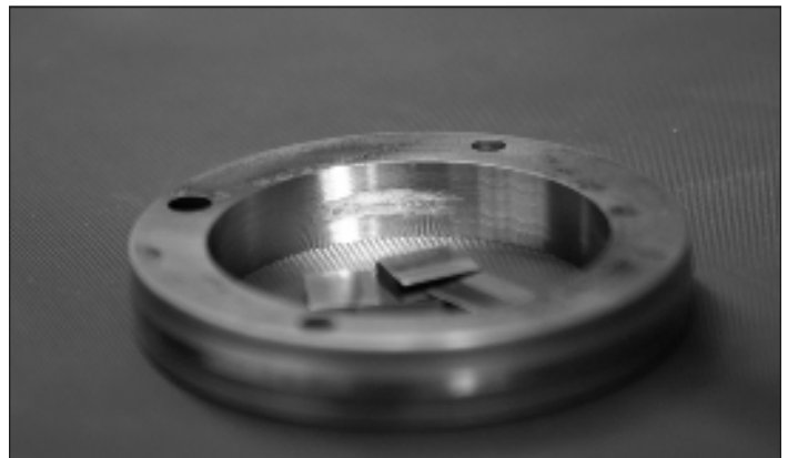
This picture shows the supply pump ring from the internal transfer pump of one of the injection pumps. It visibly shows the damage to the transfer pump liner from lack of lubrication. The transfer pump vanes are in the center of the ring and exhibited major scoring on their sides and ends, and material from the ends of the vanes can be seen transferred to the liner surface.
